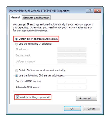
If the DHCP option is not enabled then the fix IP address set in the UC300ETH-5LPT has to be set.
