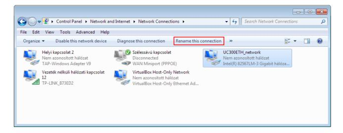
After finding and optionally renaming the connection it is time to setup the network parameters.
