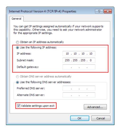
After filling the values don't forget to set the 'Validate settings upon exit' checkbox to let the parameters validate automaticaly when closing the setup. Finally press OK to all the pop up windows to exit the setup.
