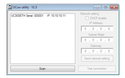
If the device of interest does not show up in the list then check the network cable connections and the router/switch device if there is any. Also check if the PC side network parameters are correct.
