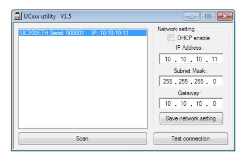
Selecting the device in the list will enable the network settings area on the screen.
