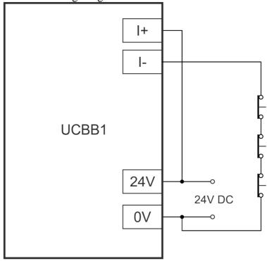
The other way is to connect the positive power supply rail (12 to 24V) to one side of the NC switch and connect the other side of the NC switch to the positive input screw terminal of the UCBB and connect the 0V to the negative input screw terminal of the UCBB. The following image shows the connection:
