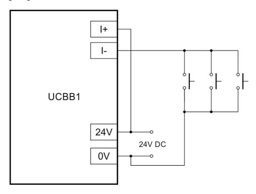
The other way is to connect the positive power supply rail (12 to 24V) to one side of the NO switch and connect the other side of the NO switch to the positive input screw terminal of the UCBB and connect the 0V to the negative input screw terminal of the UCBB.
